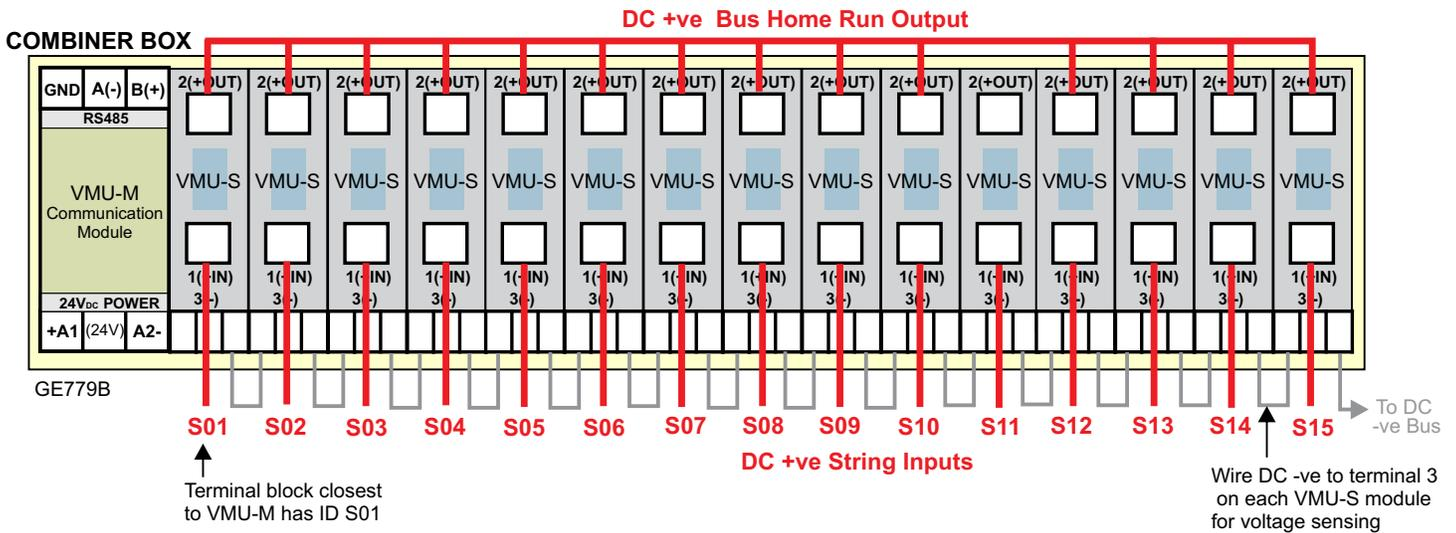
**RS485 Serial:** Each combiner will need an RS485 serial connection and 24VDC control power for the current/voltage measurement as shown in figure 4. Combiners are daisy chained together and connected to the K135 gateway in the SolarVu enclosure. Typical layout for combiners that use the CG VMU-S current/voltage sensors is shown in fig 2 and 3.
