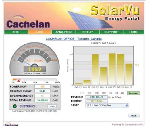
Trends are shown for the lifetime of the system using the graphs on the right. Select either an Energy or Revenue view using the button. Click the desired time period under the graph. Scroll over a data point with the mouse for more detailed information about that day. The carbon footprint pulldown gives energy equivalents for the solar power generated for the selected time period.
