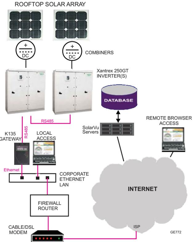
Fig 2 Schneider Xantrex 250GT RS485 Modbus serial communications
